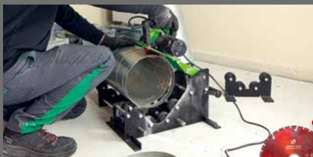
Time-saving cutting of ventilation pipes
