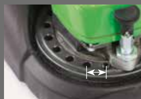
a detent point corresponds to a depth of 0.1 mm
