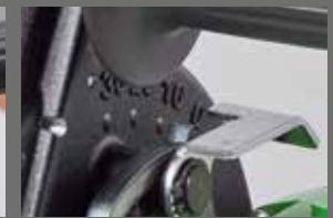
milling depth adjustment
