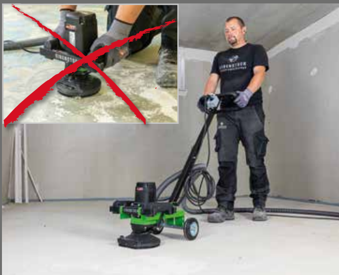
Back-friendly work with floor guide frame
