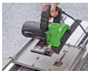
fixing of the saw without any tool
