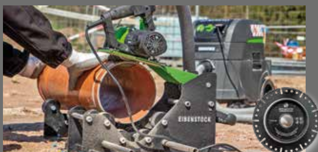
Cutting and chamfering in one operation
