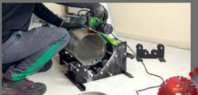
Time-saving cutting of ventilation pipes
