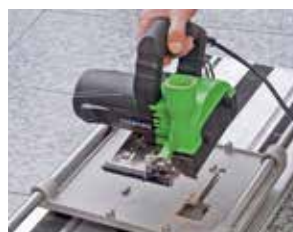
fixing of the saw without any tool
